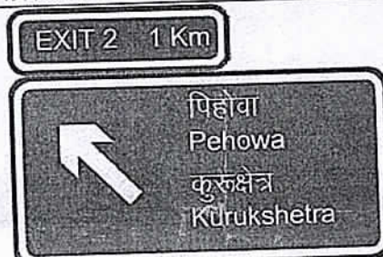
Fig 4.5 Advance Direction Sign 1 km before Exit
