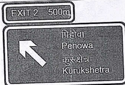
Fig 4.6 Advance Direction Sign 500 m before Exit
